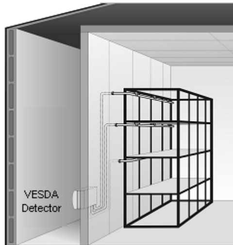
Figure 6 – Example of in-rack air sampling.
