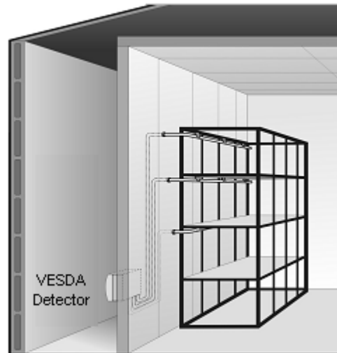
Figure 6 – Example of in-rack air sampling.
